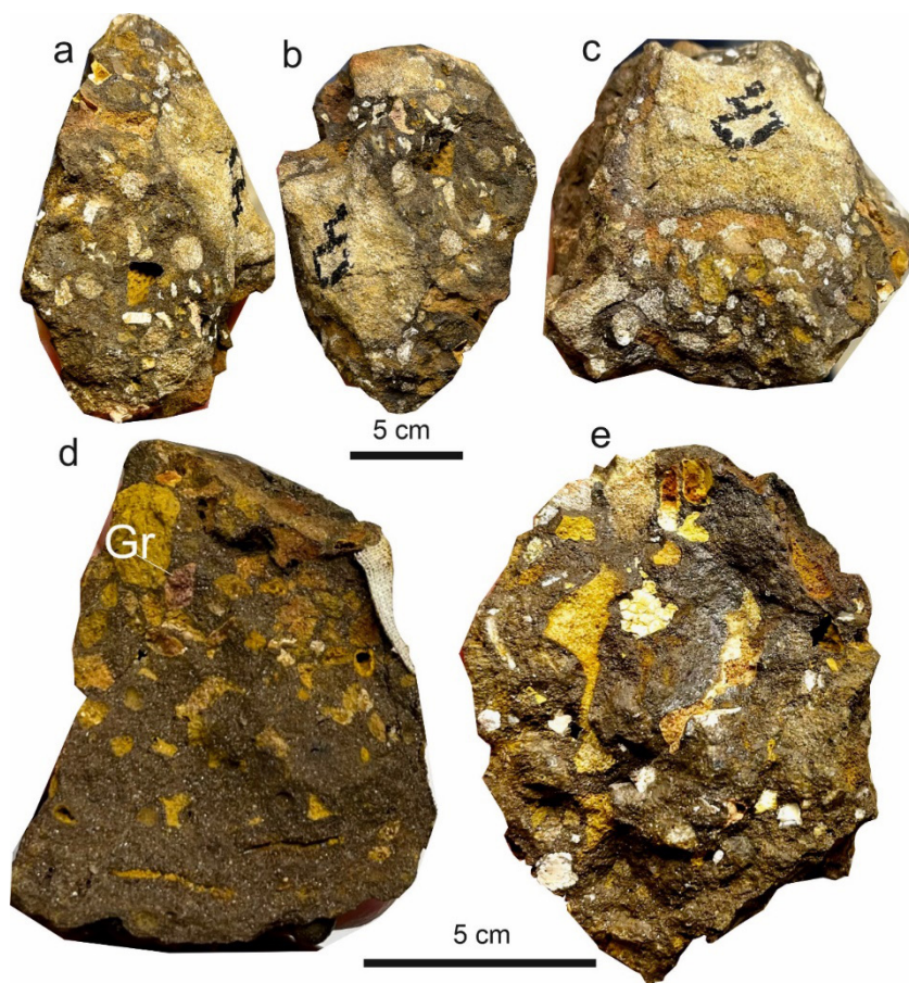
Fig. 9. Kimberlite tuff breccias with picroilmenite and pyrope (sample A74), Muaguenge area.
